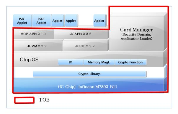
[Figure 2] Architecture of the TOE
