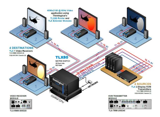
Figure 2a. Typical TOE TLX80 Matrix Switch
