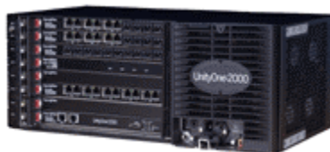
Figure 2 – UnityOne™-2000 Intrusion Prevention System (IPS)
