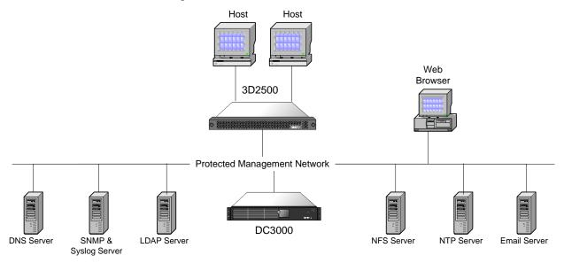
Figure 4: A DC3000 Defense Center managing a 3D2500 Intrusion Sensor deployed in inline mode (Configuration 2a)
