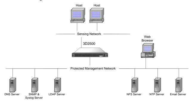
Figure 7: A standalone 3D2500 Intrusion Sensor deployed in passive mode (Configuration 3b)
