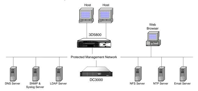
Figure 9: A DC3000 Defense Center managing a SBLinux Intrusion Sensor deployed in inline mode (Configuration 5)
