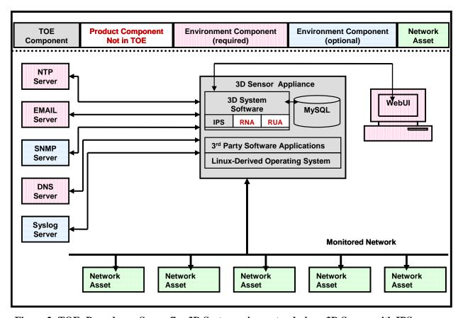
Figure 2: TOE: Boundary - Sourcefire 3D System using a stand-alone 3D Sensor with IPS
