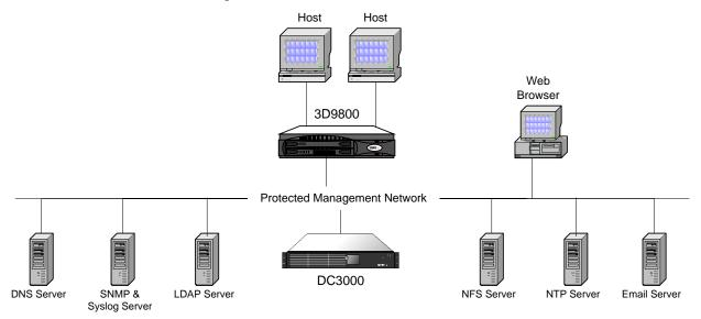
Figure 8: A DC3000 Defense Center managing a SVLinux Intrusion Sensor deployed in inline mode (Configuration 4)
