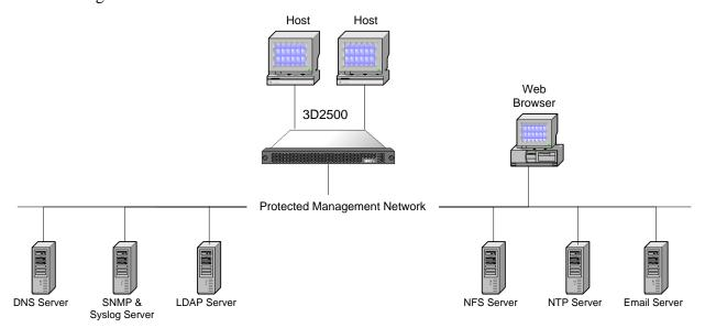
Figure 6: A standalone 3D2500 Intrusion Sensor deployed in inline mode (Configuration 3a)
