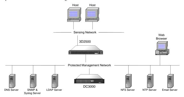
Figure 5: A DC3000 Defense Center managing a 3D2500 Intrusion Sensor deployed in passive mode
