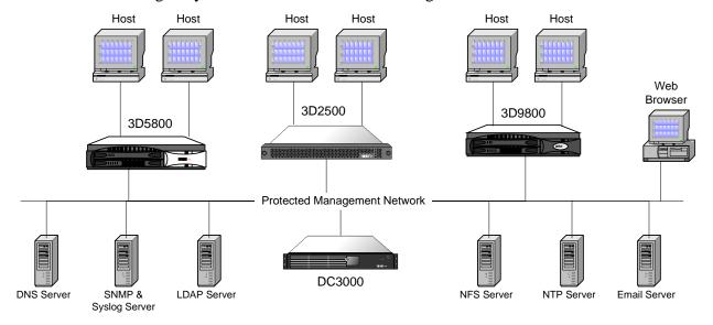
Figure 3 : A DC3000 Defense Center managing three sensors deployed in inline mode (Configuration 1)
