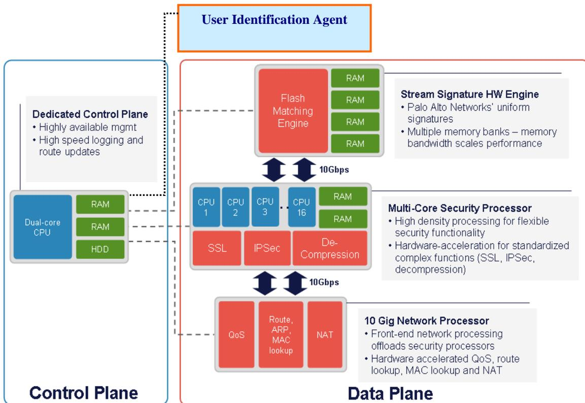
The control plane includes a dual core CPU, with dedicated memory and a hard drive for local log, configuration, and software storage. The data plane includes three components, the network processor, the security processor, and the stream signature processor (Flash Matching Engine), each with its own dedicated memory and hardware processing.
