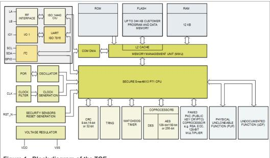
Figure 1. Block diagram of the TOE
