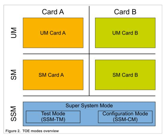
The Super-System Mode (SSM) is not available to the Security IC Embedded Software. It executes the Boot Software and Firmware.
