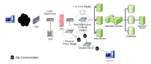
[Figure 2] WEBS-RAY V2.5(Separated Mode) Operating Environment
