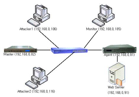
[Figure 6] Evaluator's Test Environment(Separated Mode)
