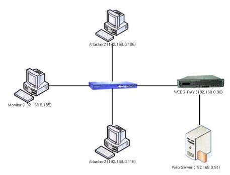
[Figure 5] Evaluator's Test Environment(Stand-alone)
