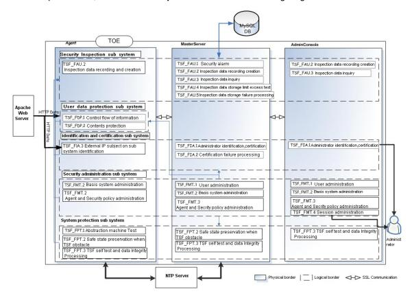
Diagram 2. 3 Physical/Logical Scope and Boundary of TOE
