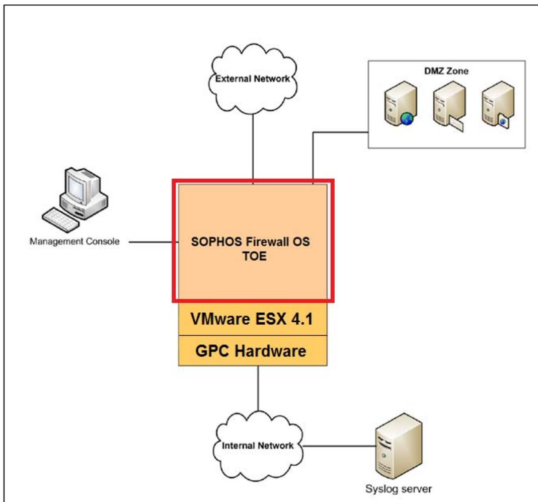
**Figure 3: TOE Physical scope and boundary on a virtual platform**
