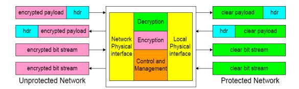
Figure 1 – Encryption data flow diagram
