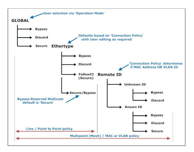
Figure 5 - Information Flow Control: Ethernet frame processing
