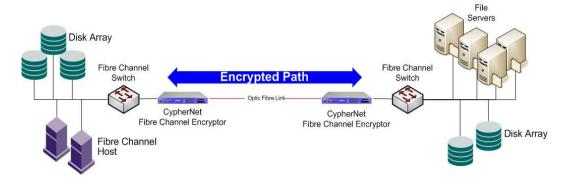
Figure 3 – Fibre Channel Security Solution
