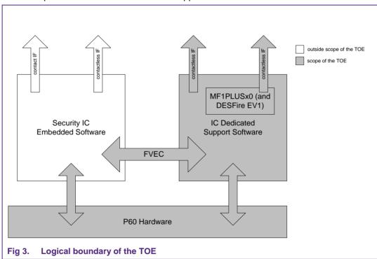
The IC Dedicated Support Software is also stored to the Test-ROM and consists of two parts.
