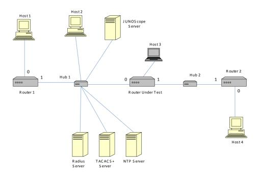
Figure 1 – Developer's Test Configuration and Evaluators' First Testing Configuration
