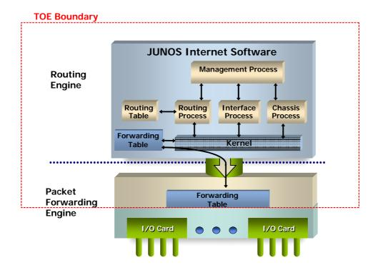
Figure 3 – TOE Architecture
