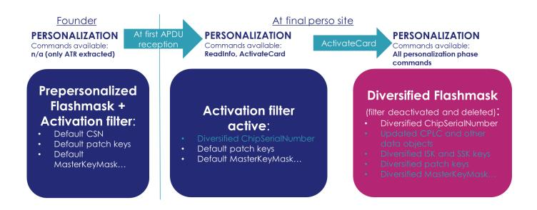
Figure 4: Delivery flow with the diversification filter mechanism
