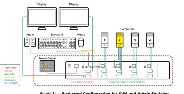
Figure 1: - Evaluated Configuration for KVM and Matrix Switches.
