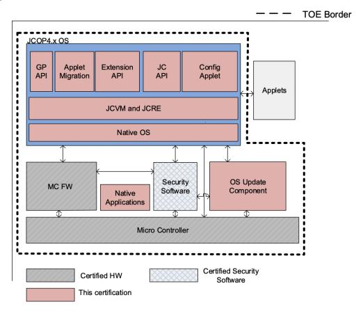
Fig. 1.1: Components of the TOE
