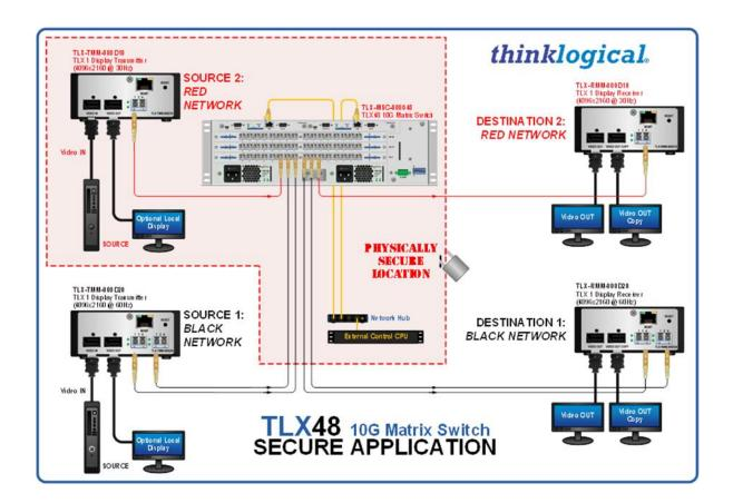
The figure shows the TLX48 Router KVM Matrix Switch in an evaluated configuration. An equivalent layout is the evaluated configuration for the TLX640 Router KVM Matrix Switch.
