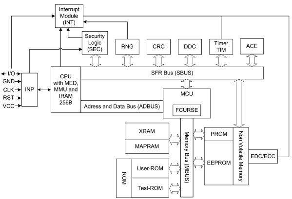
Figure 1: Block diagram of the TOE
