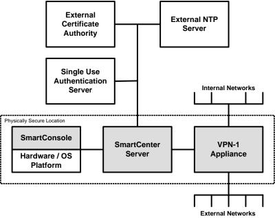
Figure 1 - TOE Hardware Components
