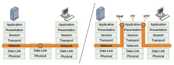
Figure 2-5- Traffic filtering (left) vs. Application-level Proxies
