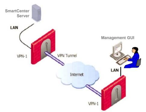
In both configurations, TOE evaluated configuration guidance requires the administrator workstation to be deployed on a protected subnet that is directly connected to a TOE Check Point VPN-1/FireWall-1 NGX (R60) appliance. The appliance protects the workstation from any network access by untrusted entities. The workstation operating system and hardware do not contribute any security functionality, and are considered to be outside the boundaries of the TOE.
