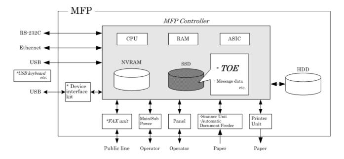
Figure 2 Hardware composition relevant to TOE
