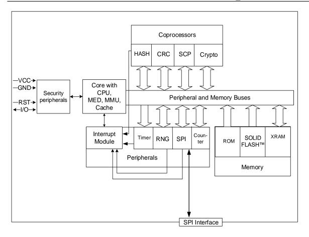
Figure 1: Block diagram of the SLI9670\_2.0
