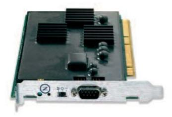
In addition to the PCI connection to a server, the HSM also supports a connection to a smart card reader. Smart cards may be used to hold logical tokens used to encrypt key blobs. Possession of the correct smart card provides authorization to use the stored key.
