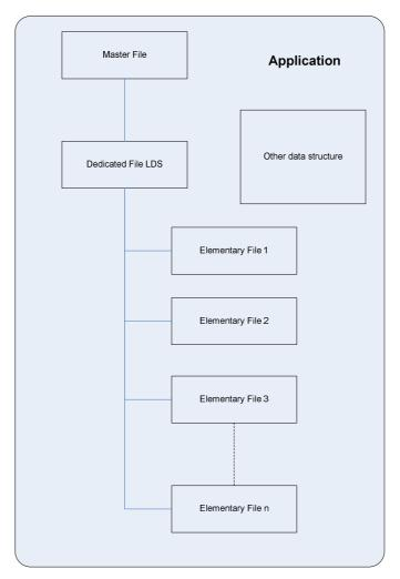
Figure 3 : Structure of the file system
