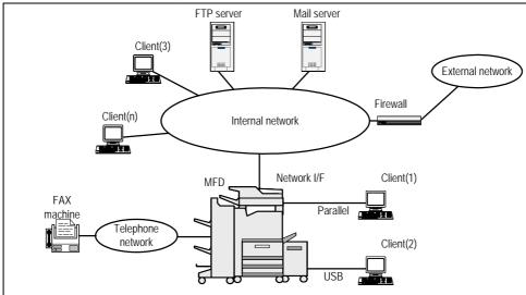
Figure 3: Usage environment of the TOE
