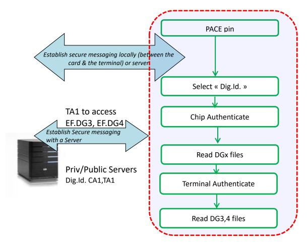
A Card can have an MRTD instance of the eTravel Application and/or a second instance dedicated to the Digial Identity in order to identify a citizen with its user consent. In this part, we will focus only on the Digital Identity part. The LRTD is defined in the chapter 2.3.3 of the
