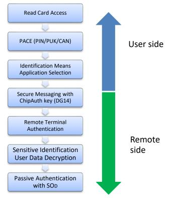
Figure 2: Remote Inspection Procedure
