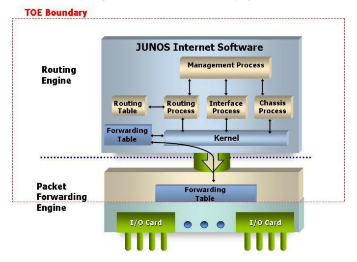
The interfaces to the TOE are twofold: the routing interfaces (including control traffic) and the management interfaces. The management interfaces include the TOE console interface through which the appliance can be managed locally, the dedicated management ethernet interface and the in-band management interface via the
