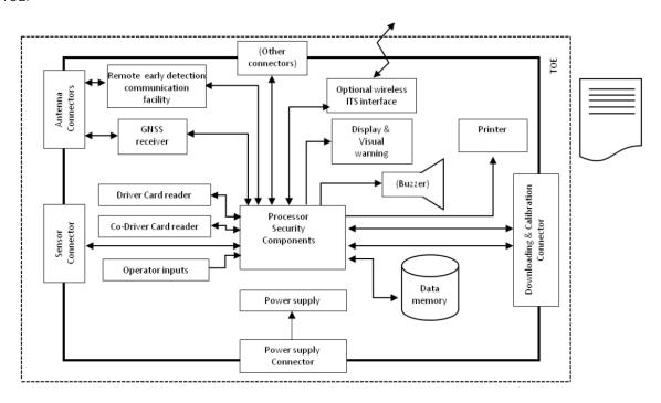
Figure 1-1 Configuration 1: Internal GNSS receiver and internal remote early detection communication facility
