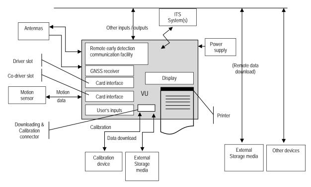
Figure 1-4 VU operational environment (internal remote early detection communication facility / internal GNSS receiver)
