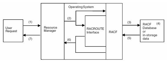
Figure 1: RACF and its relationship to the operating system
