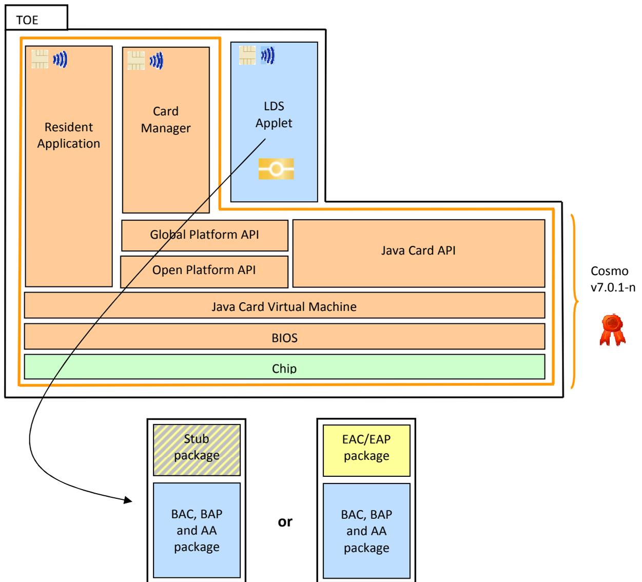
**Figure 1 TOE architecture**
