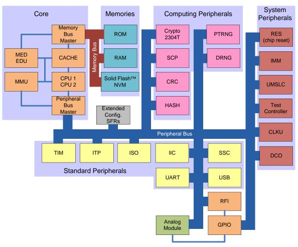
Figure 1: Block diagram of the TOE
