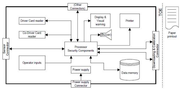
Figure 1: Simplified Drawing of the VU
