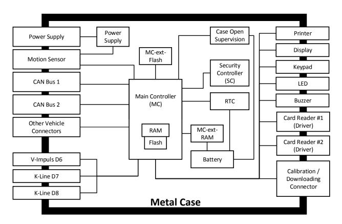
Figure 4: EFAS-4.8 V03.50 with Interfaces
