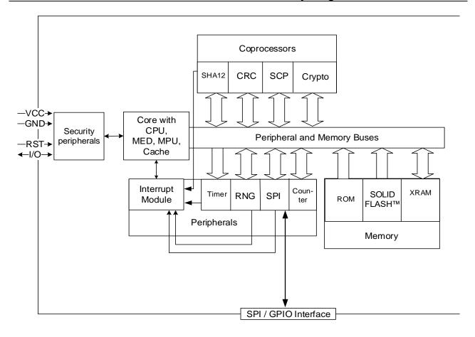
Note: The SLB9672\_2.0 v16 includes an SPI interface, the SLB9673\_2.0 v26 includes an I2C interface.
