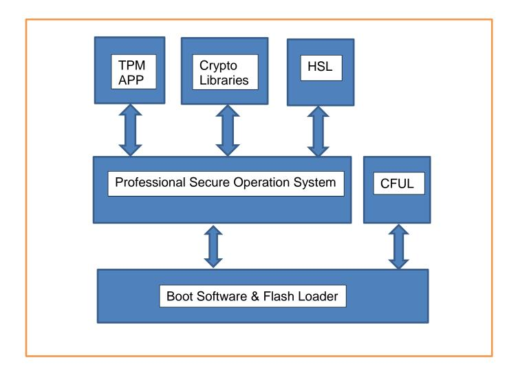
Figure 2: Firmware block diagram of the TPM
