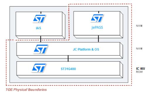
The TOE is a contact/contactless chip and comprises the following elements:
