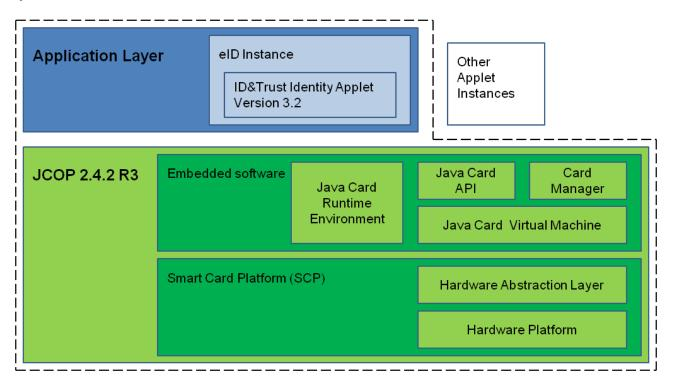
Figure 1 – The logical architecture of the TOE
