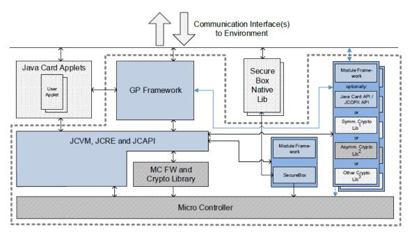
Figure 1 Logical architecture of the TOE
