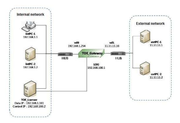
(Figure 4) Evaluator's test configuration
