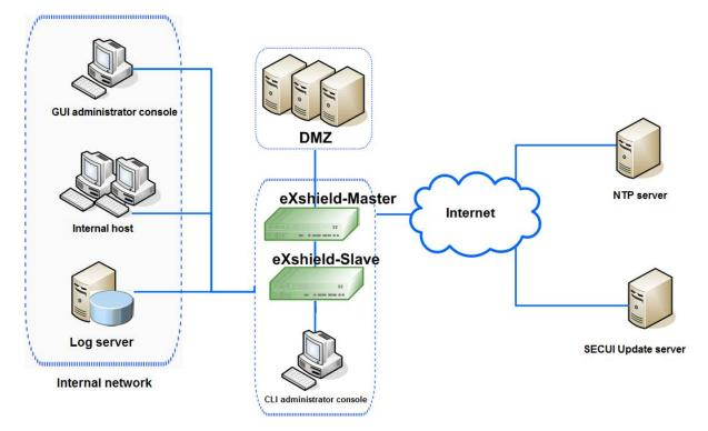
Figure 2-2 Configuration of eXshield Security Switch V1.0: 2
