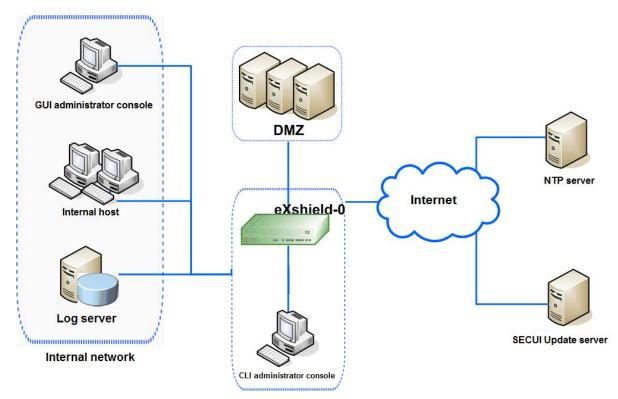
Figure 2-1 Configuration of eXshield Security Switch V1.0
