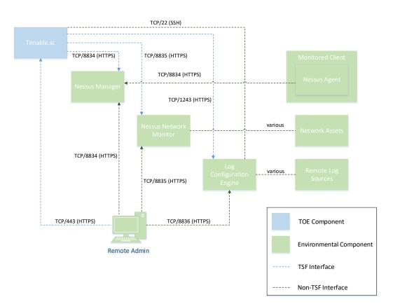
Figure 1 – Example Deployment
