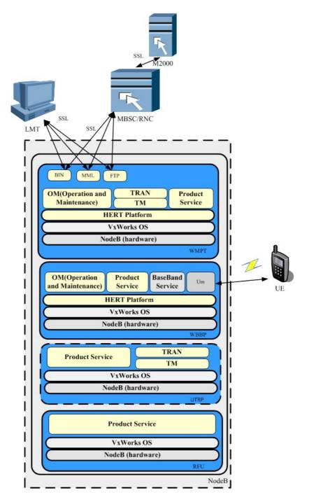
In the above diagram, the blue areas are parts of the TOE. NodeB includes Operation and Maintenance (OM), Baseband Service, and HERT platform.
