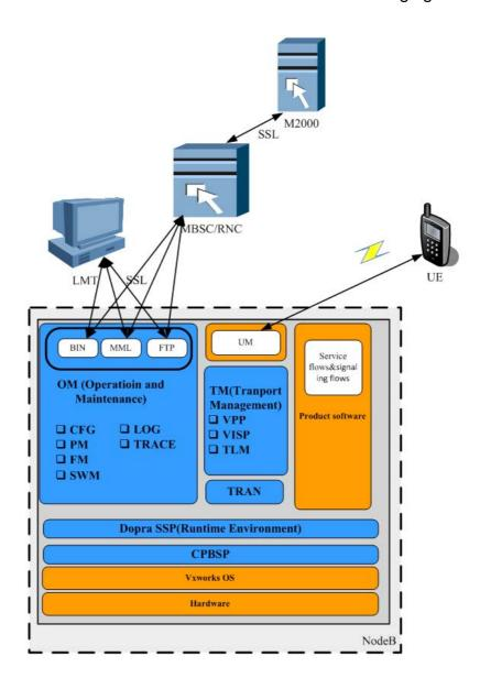
The TOE is pure software. OS and other software provided by particular products is TOE environment.
