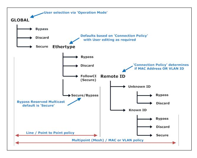
Figure 5 - Information Flow Control: Ethernet frame processing
