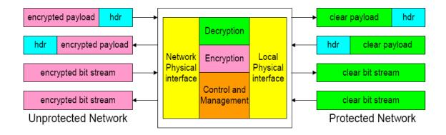
Figure 1 – Encryption data flow diagram
