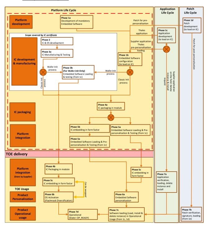
Figure 5: Manufacturing phases description
