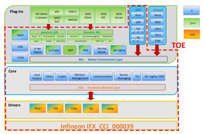
Figure 1: MultiApp V5.0.A smartcard architecture
