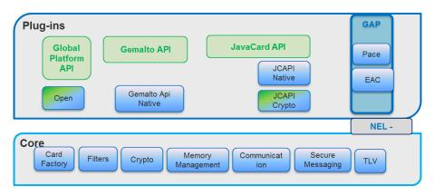
Figure 2: MultiApp V5.0.A Java Card platform architecture
