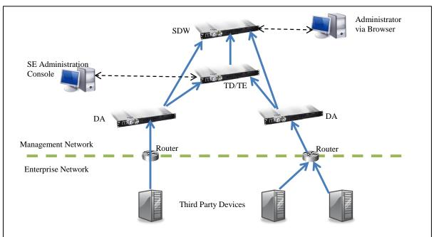
A diagram of the Trustwave SIEM Enterprise Version 2.3.3 architecture is as follows:
