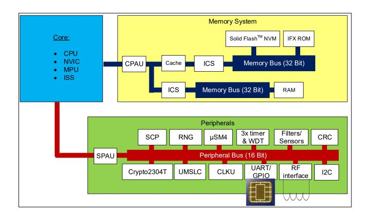
The TOE hardware consists of a core, a memory system and peripherals.
