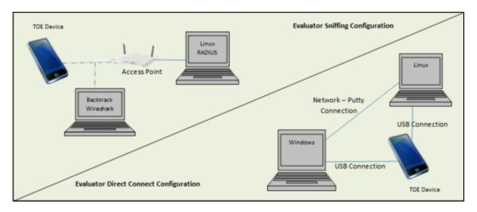
Figure 1 Evaluator Test Setup
