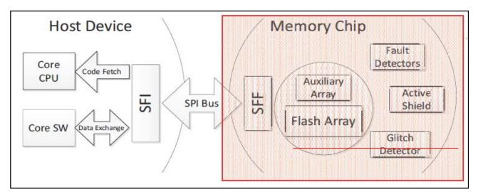
Figure 1 TOE Architecture
