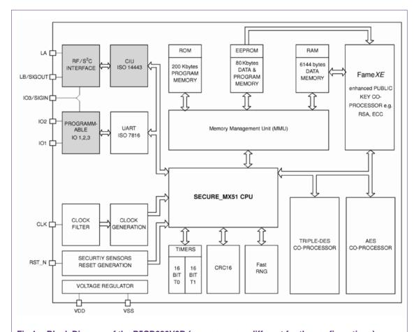
Fig 1. Block Diagram of the P5CD080V0B (grey areas are different for the configurations)
