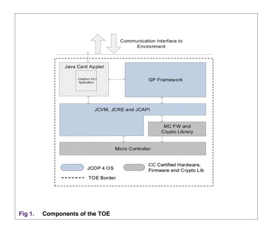
The TOE consists of an applet which is executed by a software stack that is stored on a Micro Controller. For a complete picture of the TOE see Fig 1, and for details with regards to the different components see section 1.3.5.
