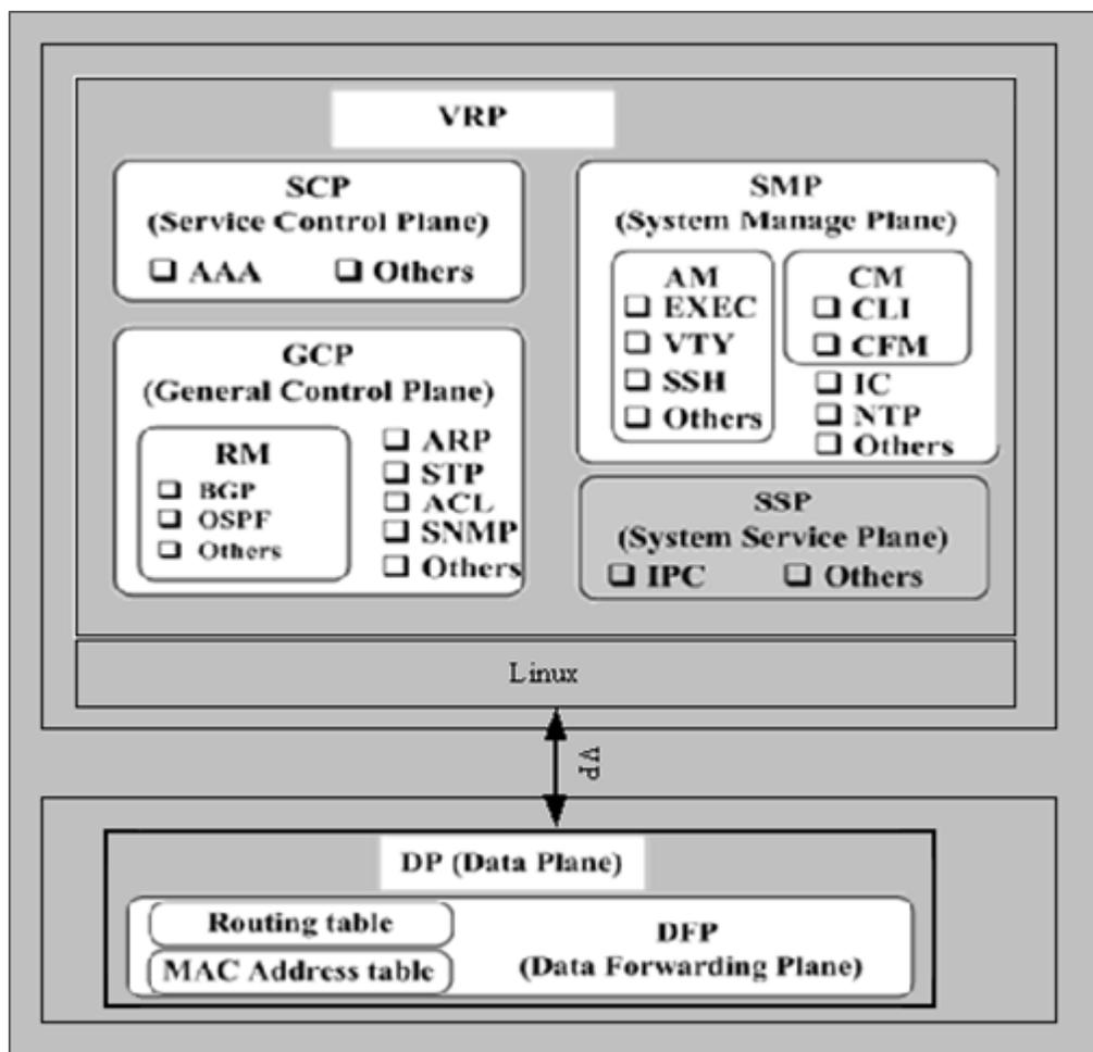
Figure 3: TOE Software architecture
