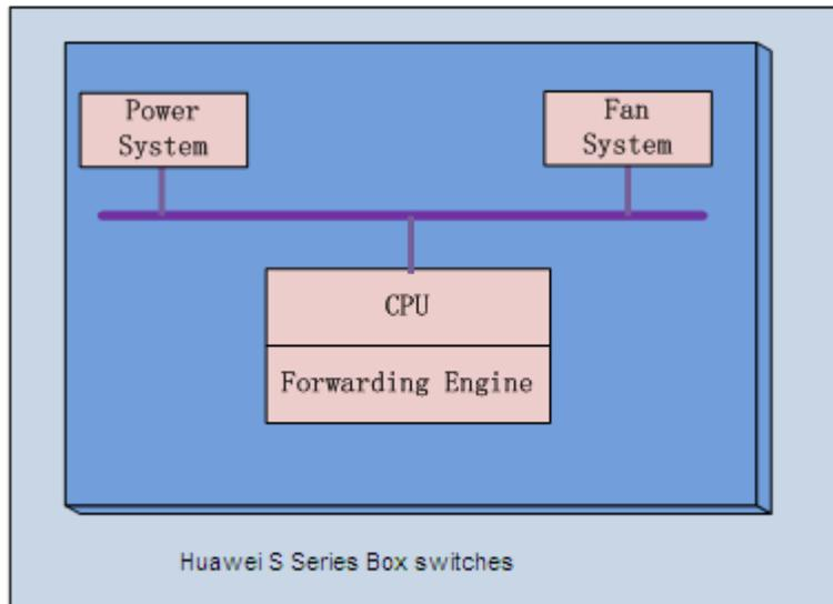
Figure 2: TOE Physical Architecture of Box Switch
