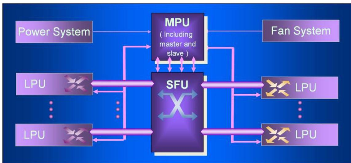
Figure 1: TOE Physical architecture of Chassis Switch
