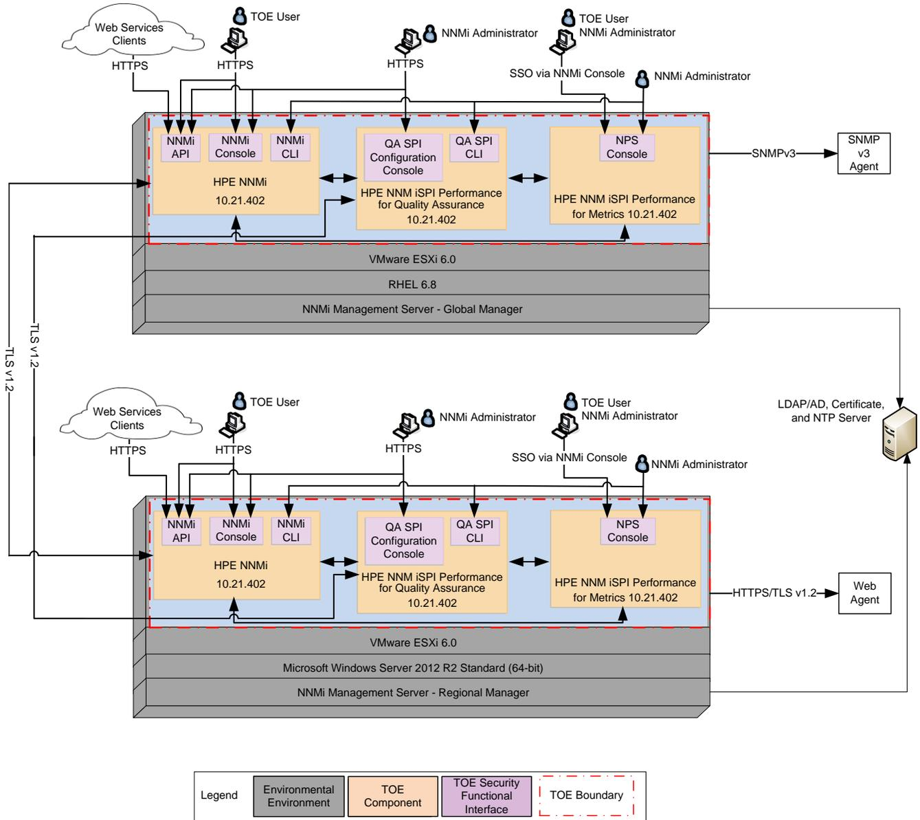
**Figure 2 – Evaluated Configuration of the TOE**
